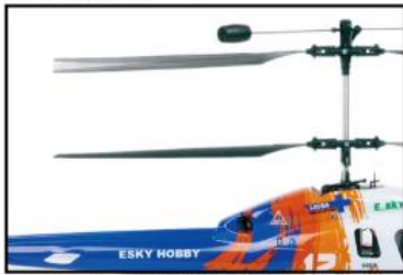
Main blades are not tracking in the same plane 主旋翼旋转不在同一平面
