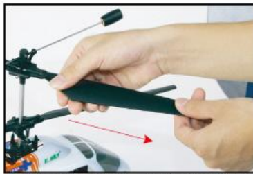
用左手抓住桨的根部，用右手捏住桨叶由里向外滑动，重复此动作。Please adjusting the main blade like this way until the tips are tracking in the same plane
