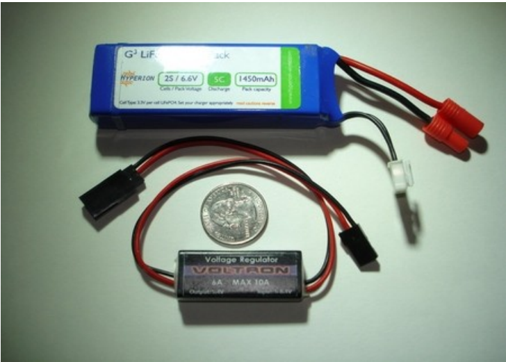
Picture 1: Voltage regulator size compared to a quarter and a 1450mAh LiFe 2S Hyperion battery pack. Also see a pic of the backside of the regulator at the end of this report.
