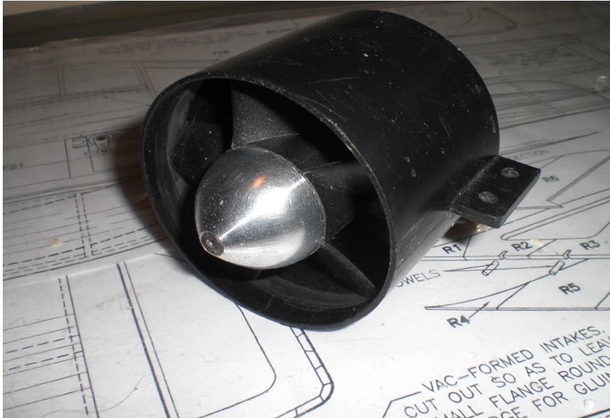
Illustration 5: A wemotec 70mm 5-bladed fan with Mega-EDF motor fitted
